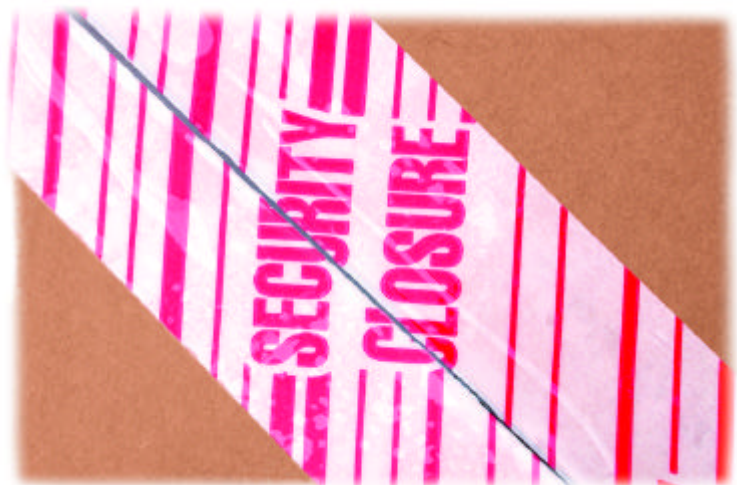
Box sealed with 1248, cut and resealed with clear acrylic tape
